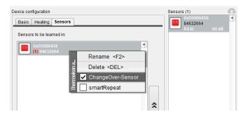
Sensors and devices, within range, are listed on the right side of airConfig. To learn in a specific sensor simply drag and drop the (activated) symbol into the sensors input tab of the STC-DO. The Sensor's (EEP) type must be known to be assigned correctly through activation of the sensor or switch. The sensor type is coded in the EEP, which is included in the sensor's LRN telegram.
