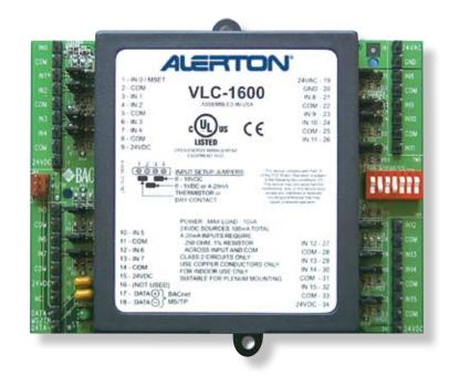
TheAlerton<sup>®</sup> BACtalk<sup>®</sup> VLC-1600 is a high-performance, fully programmable input monitoring device. With 16 high-resolution inputs, it is perfectly suited for applications with high input density, where it can augment the input capabilities of other controllers. The VLC-1600 has no control outputs. As a native BACnet controller, it integrates seamlessly with your BACnet system, communicating on a BACnet MS/TP LAN at up to 76.8 Kbps.
